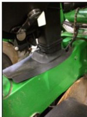
Incorrectly Installed Boot
