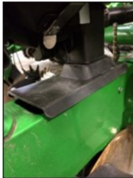
Correctly Installed Boot
