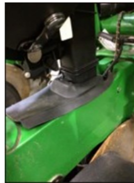
Incorrectly Installed Boot
