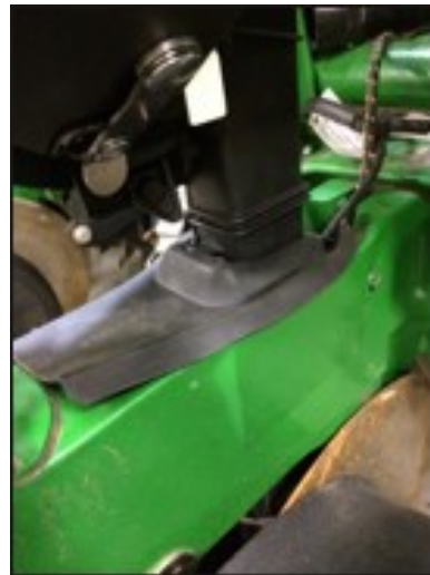
Incorrectly Installed Boot
