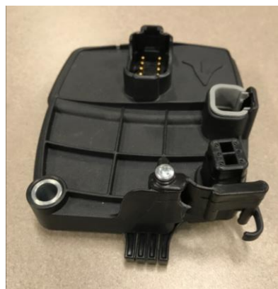
Align Latch Replacement in place of broken latch and insert screw.
