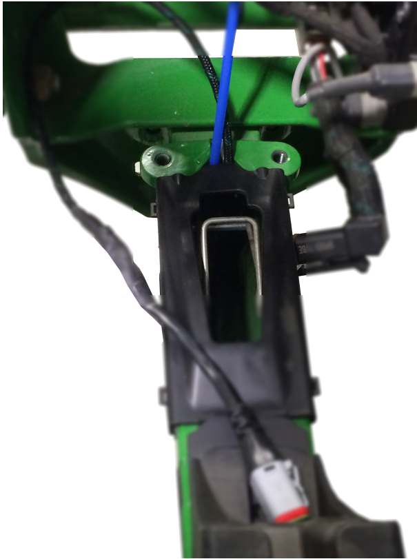
Harness routed in front of Seedtube
