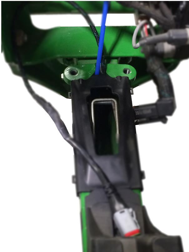
Figure 1. Harness routed in front of Seedtube
