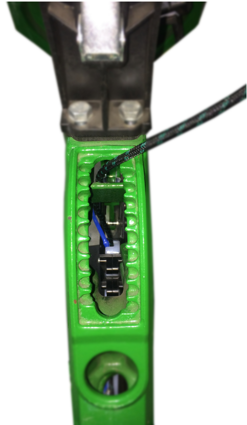
Figure 2. Harness routed out depth adjustment
