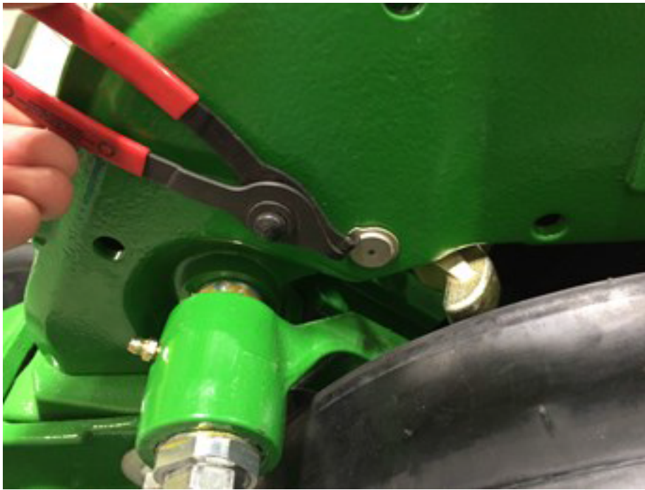
c: Secure the load cell with the supplied snap ring.
