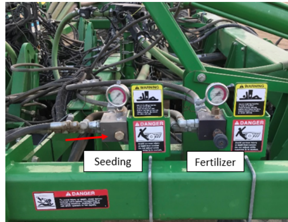
Figure 5. Three Frame Section Hydraulic Block
