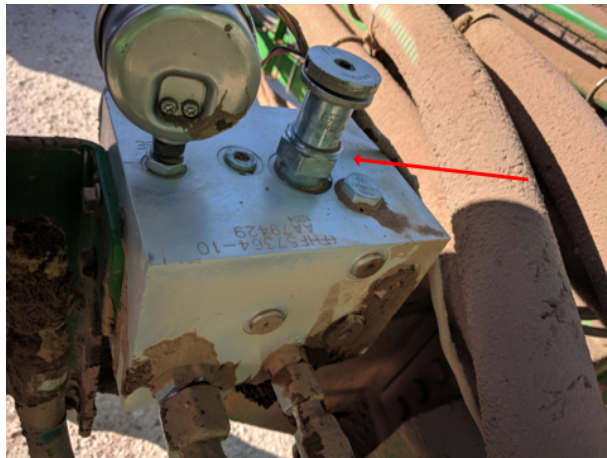
Figure 4. Five Frame Section Hydraulic Block
