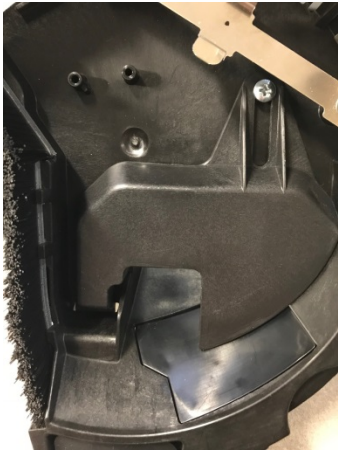
Existing baffle to be removed
