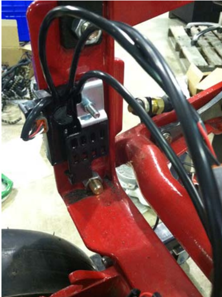
RUM installed on White 9000-series row unit
