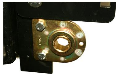
Hex Shaft Bearing Shown as installed onto the Base Mount, directly under the Arm Mount.
