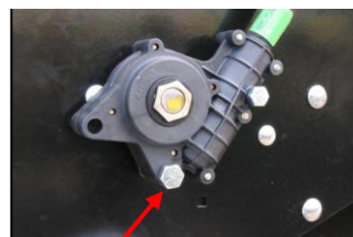
3/8" X 2" Bolt Fixes the Driver Gear Box in Place
