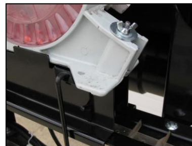
8000 Series White Meter Uses a 5" J-Bolt to secure it to the boot
