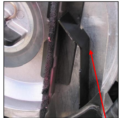
Less Than .060" Gap Between Riser of Seed Boot and Meter Housing
