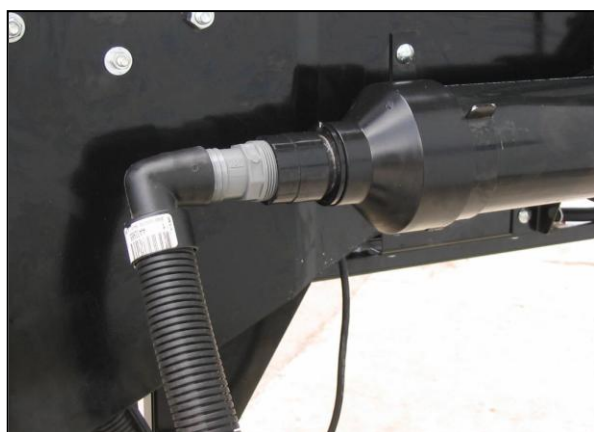
3" Flexible Hose Connected to Meter Air Inlet.
