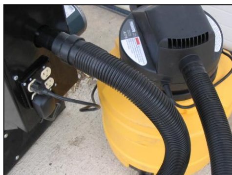
Shop Vac Setup to Supply Air to the White Meter (Hose connected to blower port)
