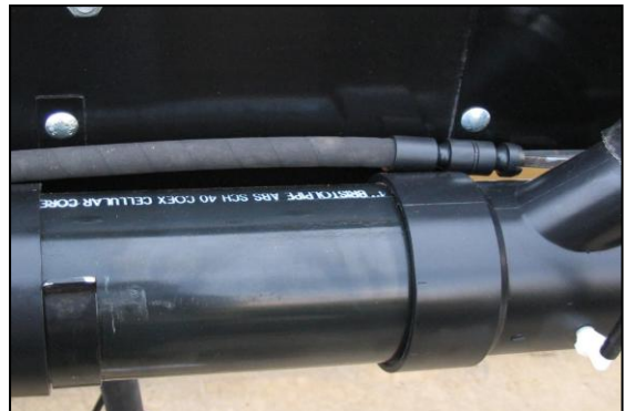
Rest Cable on Air Accumulator When Not in Use
