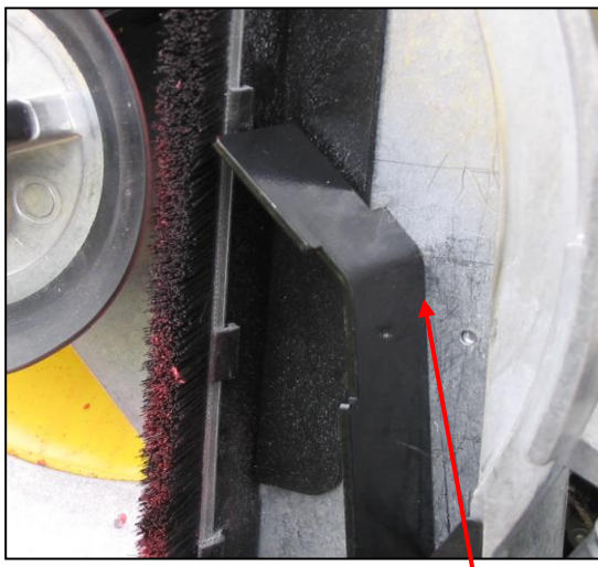
Less than .060” Gap Between Riser of Seed Boot and Meter housing
