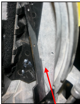
Less than .60" gap between riser of seed boot and meter housing
