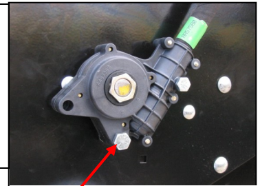
5/16" X 2-1/4" Bolt Fixes the Driver Gear Box in Place
