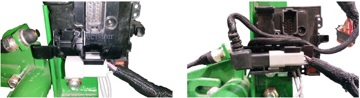
Illustration 18 – Row Harness and Y-Harness Connected
