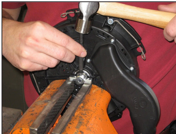
Figure 2: Driving Out Spring Pin
