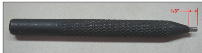
Figure 1: 3/32" Diameter Punch Shortened to 1/8" Length
