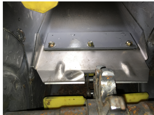
Figure 8. Center Divider Repair Kit and Divider Installed
