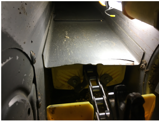
Figure 1. Example of a Broken Divider
