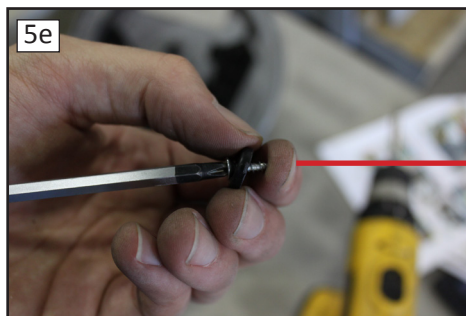
Insert Screw D (#6 Flat Hi-Lo) into the shim washer.
