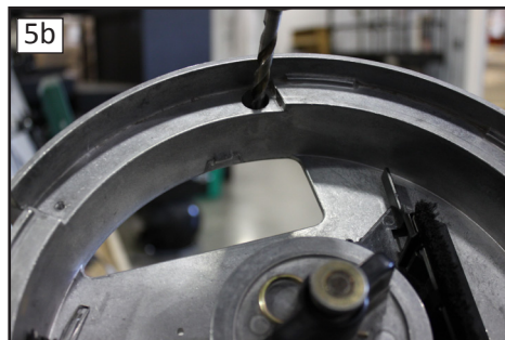
Drill a \frac{5}{16} " hole at the large Singulator hole.
