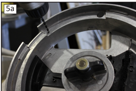
Drill a \frac{1}{8} " hole at the small Singulator hole.
