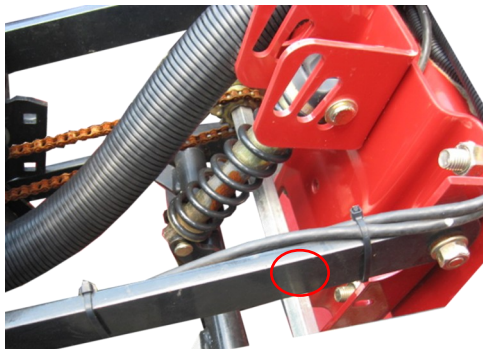
OEM parallel arms lacking a pre-drilled holes for mounting air spring brackets.
