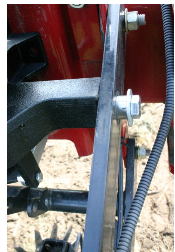
14" CNH Upper Parallel Arm replacements compatible with mounting of air spring brackets.
