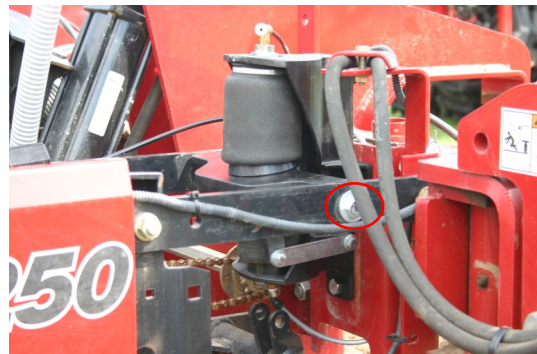
14" CNH Upper Parallel Arm replacements compatible with mounting of air spring brackets.
