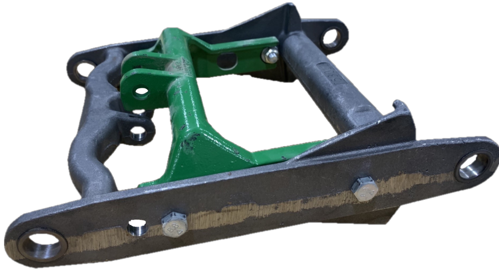
Figure 4. JD Bracket (Green) installed on Durawear short arms (Grey)
