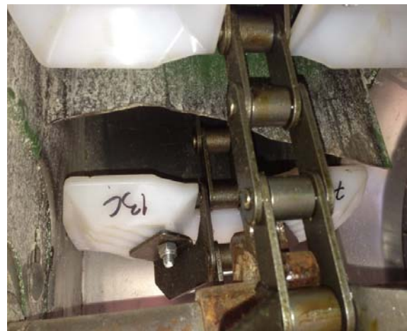
BROKEN DIVIDER PLATE CAN BE A CATCH POINT FOR PLASTIC PADDLES.
