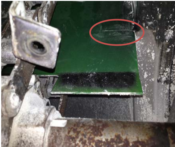
LOOK FOR CRACKS IN THE DIVIDER PLATE. THESE SHOULD BE WELDED.
